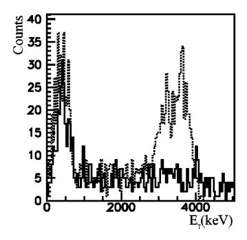
Figure 2.5: Measured  $\gamma$ -ray energy spectrum from experiment for  $^{24}$ O (solid line) and a simulated (dashed)  $\gamma$ -ray energy peak [21]. The  $\gamma$ -ray peak was simulated with an energy of 3.7 MeV assuming 20% of the  $^{24}$ O is produced in the  $2_1^+$  state. The lower limit of the production to the  $2_1^+$  state based on the data was 3%.
