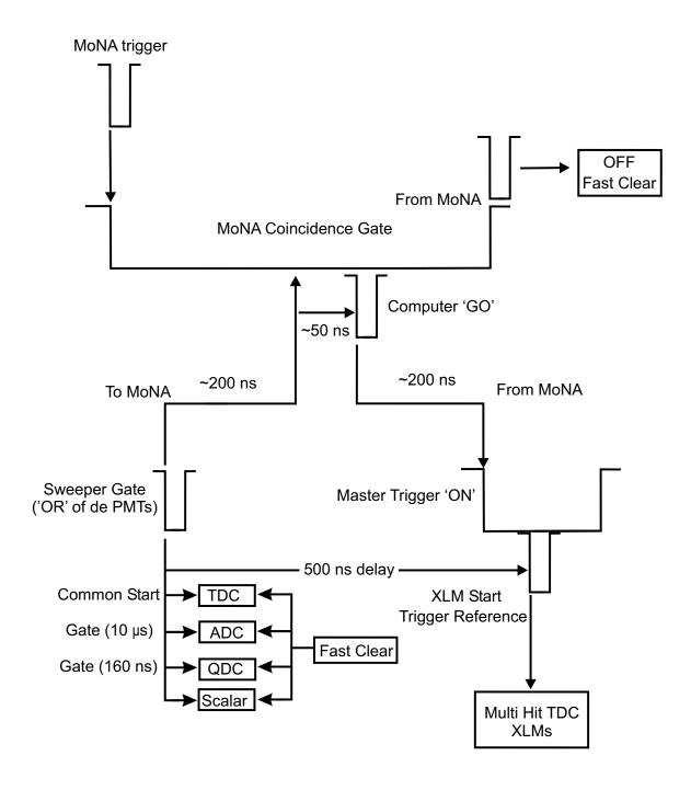
Figure 3.11: Charged particle trigger
