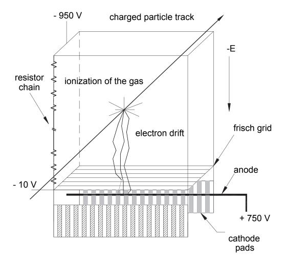
Figure 3.8: Cathode readout drift chamber
