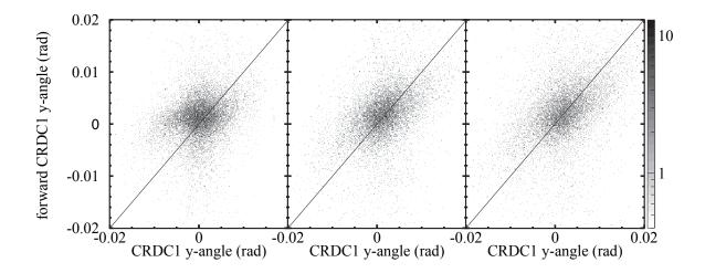
Figure 4.35: Forward-tracked CRDC1 y-angle versus measured CRDC1 y-angle. Low  $B\rho$  setting (left), data-taking  $B\rho$  setting (center), and high  $B\rho$  setting (right).
