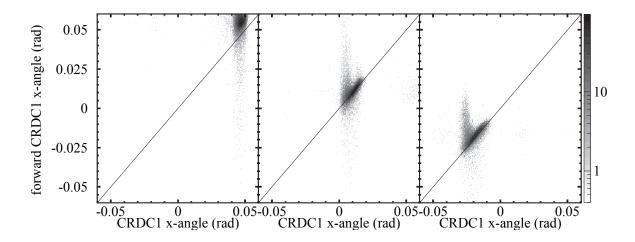
Figure 4.33: Forward-tracked CRDC1 x-angle versus measured CRDC1 x-angle. Low  $B\rho$  setting (left), data-taking  $B\rho$  setting (center), and high  $B\rho$  setting (right).
