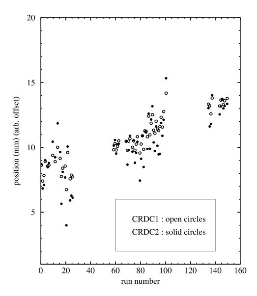
Figure 4.5: Mean y-position of both CRDCs versus run number for all charged fragments in coincidence with incoming  $^{26}$ Ne secondary beam. The arbitrary offset is for display purposes.
