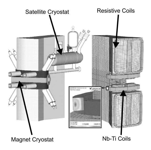
Figure 3.7: Sweeper Magnet technical drawings  $\,$
