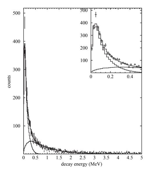
Figure 5.2: Decay energy spectrum of  $^{23}\text{O}^*$ . The upper histogram is the result of a simulation including contributions from a resonant state ( $E_r = 45 \text{ keV}$ ,  $\Gamma = 20 \text{ keV}$ , middle histogram) and background with a thermalized neutron source (lower histogram).
