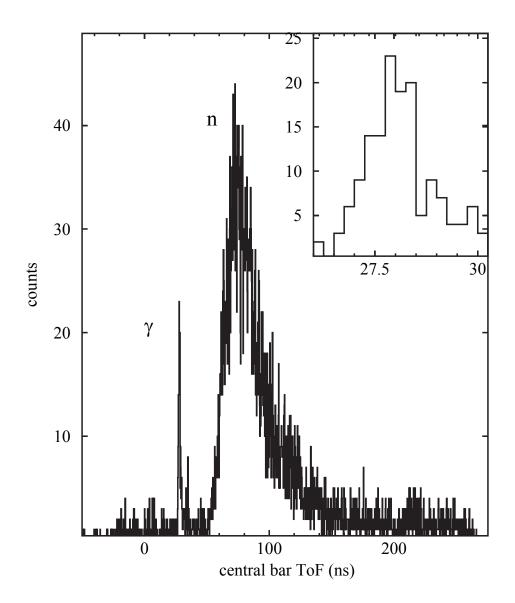
Figure 4.28: Prompt  $\gamma$ -ray and neutron peaks in the neutron ToF spectrum. The high yield of prompt  $\gamma$ -rays was produced using a thick reaction target. The upper-right insert is zoomed in on the prompt  $\gamma$ -ray peak.
