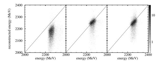
Figure 4.39: Backward reconstructed secondary beam energy versus measured secondary beam energy. Low  $B\rho$  setting (left), data-taking  $B\rho$  setting (center), and high  $B\rho$  setting (right).
