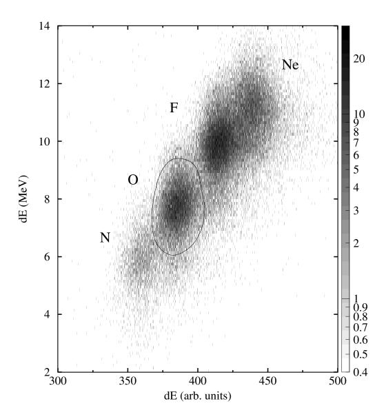
Figure 4.17: Energy loss (ionization chamber) versus energy loss (dE scintillator). The cut for oxygen isotopes is shown by the curve.
