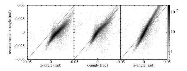
Figure 4.36: Backward reconstructed target x-angle versus measured target x-angle. Low  $B\rho$  setting (left), data-taking  $B\rho$  setting (center), and high  $B\rho$  setting (right).
