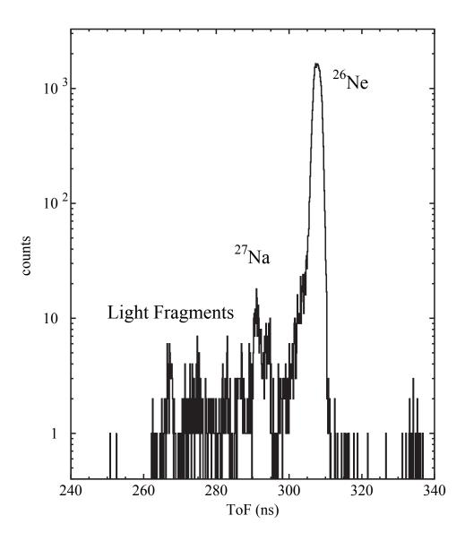
Figure 4.3: Time-of-Flight (ToF) secondary beam identification plot
