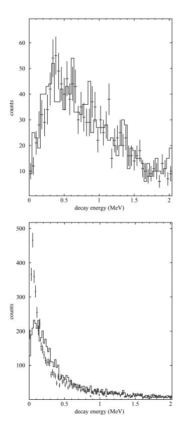
Figure 4.43: Decay energy spectra for correlated (points with error bars) and uncorrelated (histogram) neutron and charged fragment events for  $^{22}\mathrm{O}^*$  (top) and  $^{23}\mathrm{O}^*$  (bottom).
