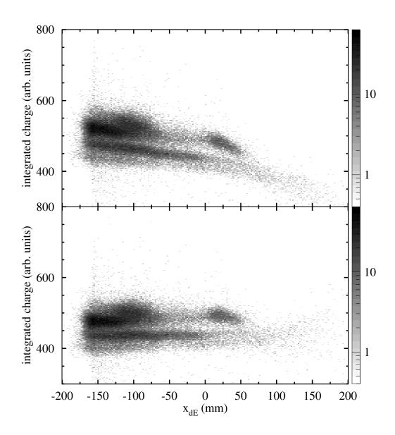
Figure 4.15: Down-right PMT integrated charge versus  $x_{dE}$ . No position correction (top) and with position correction (bottom) using the  $x_{dE}$  parameter.
