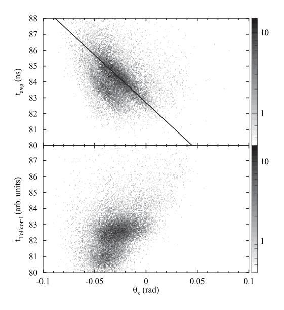
Figure 4.20: Average ToF versus  $\theta_x$  without (top) and with (bottom)  $\theta_x$  correction. The line in the upper spectrum indicates the corrected trend.
