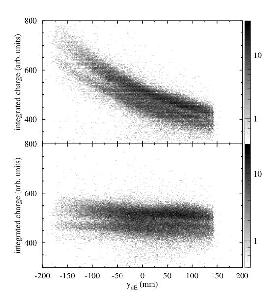
Figure 4.14: Down-right PMT integrated charge versus  $y_{dE}$ . No position correction (top) and with position correction (bottom) using the  $y_{dE}$  parameter.
