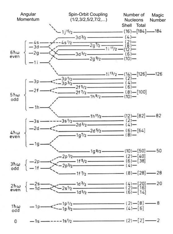
Figure 1.2: Schematic plot of energy levels in the nuclear shell model adapted from Reference [9]. The first column lists the principle angular momenta levels from the harmonic oscillator potential, the second column includes the spin-orbit potentials, the third column labels the sub-shell and total occupancy, and the last column represents the magic numbers.
