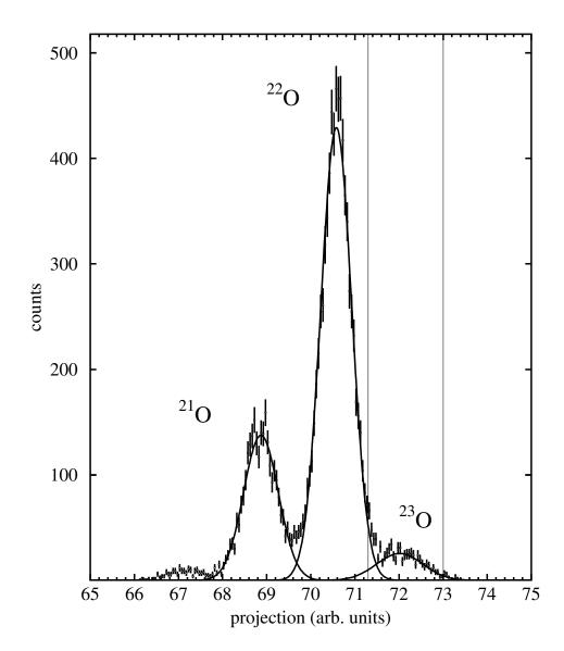
Figure 4.27: Projection from TKE versus corrected ToF plot where the solid lines represent Gaussian fits of the  $^{21,22,23}$ O isotopes. The reduced  $\chi^2$  of the nine parameter fit is 1.257.
