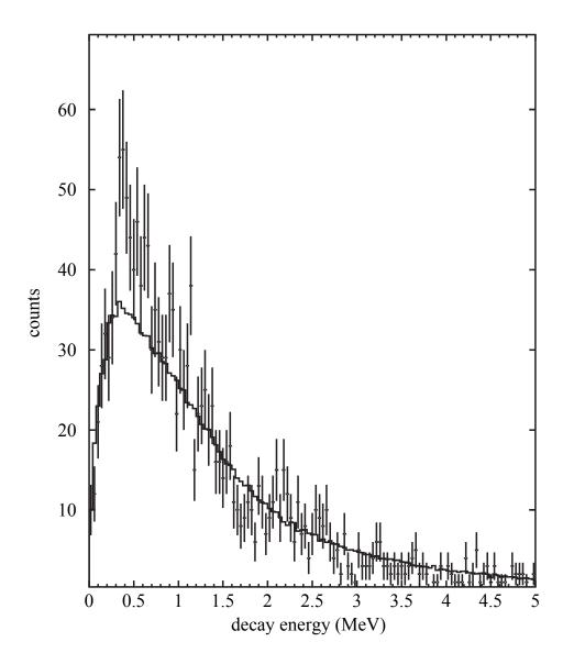
Figure 5.1: Decay energy spectrum of  $^{22}\mathrm{O}^*$ . The histogram corresponds to fit assuming a thermalized neutron source of nuclear temperature T=2 MeV.
