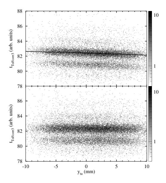
Figure 4.23: Corrected ToF  $t_{\rm ToFcorr3}$  versus y-position at the reaction target uncorrected (top) and corrected (bottom).
