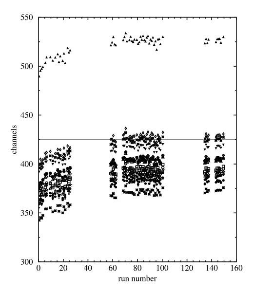
Figure 4.12: Ionization chamber pad peaks versus run number. The symbols represent each pad used from the ionization chamber.
