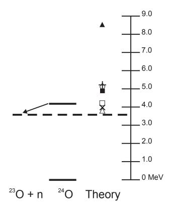
Figure 5.8: Comparison of theory to the extracted decay energy (solid line) for the first unbound excited state of  $^{24}$ O. Theoretical calculations  $\triangle$ : Obertelli [27],  $\times$ : Khan [23],  $\square$ : Siiskonen [25],  $\blacksquare$ : Volya [26],  $\diamond$ : Utsuno [24], +: Brown [28],  $\blacktriangle$ : Thiamova [22]. The dashed line marks the one-neutron separation energy of 3.61 MeV  $^{24}$ O.
