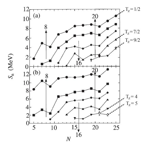
Figure 2.4: One neutron separation energy  $(S_n)$  versus neutron number (N) for odd N, even Z (a) and odd N, odd Z (b) adapted from Reference [19]. The lines connect points with the same  $T_z$  values, which are noted to the side for clarity.
