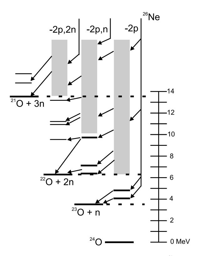
Figure 5.4: Separation energies of three-, two-, and one-neutron relative to <sup>24</sup>O calculated using Reference [29]. The gray boxes represent a continuum of unbound states, the dashed lines indicate three-, two-, and one-neutron separation energy relative to <sup>24</sup>O, the thick solid lines represent predicted unbound states, and the thin solid lines are measured excited states. The arrows indicate possible paths for producing neutrons with a charged fragment.
