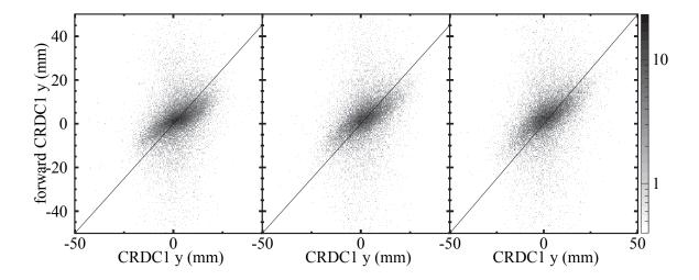
Figure 4.34: Forward-tracked CRDC1 y-position versus measured CRDC1 y-position. Low  $B\rho$  setting (left), data-taking  $B\rho$  setting (center), and high  $B\rho$  setting (right).
