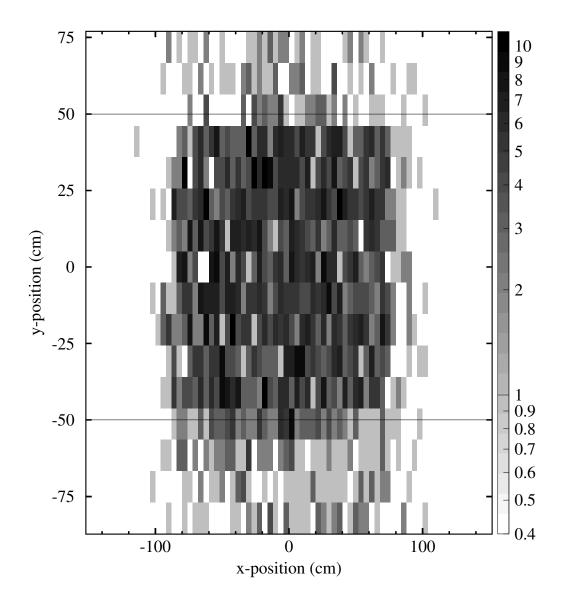
Figure 4.29: y-position versus x-position on MoNA. The lines are drawn to indicate the vertical acceptance due to the opening at the end of the Sweeper Magnet.
