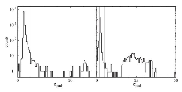
Figure 4.6: Pad width  $\sigma_{pad}$  for CRDC1 (left) and CRDC2 (right). The events between the lines in each spectrum were accepted for the next cut for each CRDC separately.
