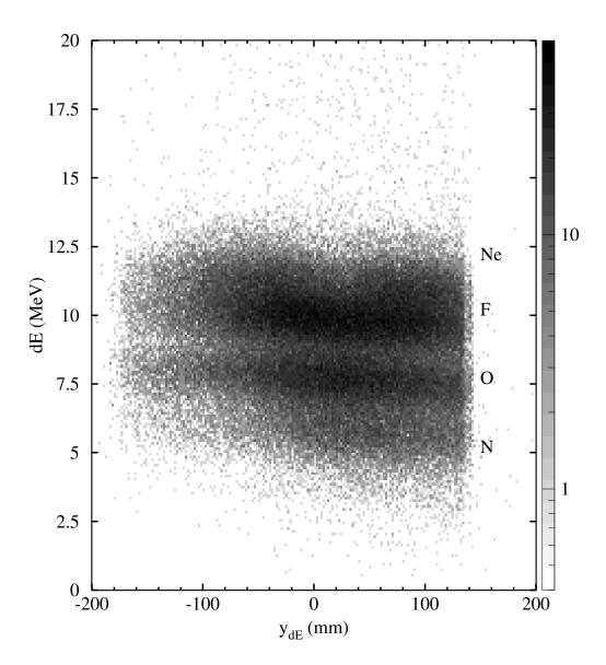
Figure 4.13: Energy loss in ionization chamber versus vertical position at the dE scintillator  $(y_{dE})$ .
