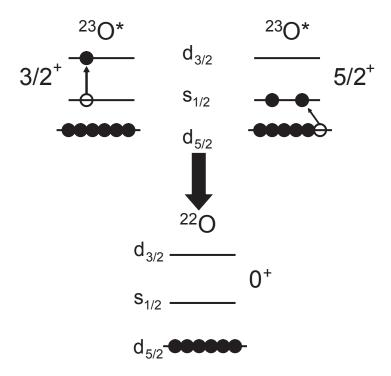
Figure 5.5: Single particle configurations for  $5/2^+$  and  $3/2^+$  unbound states in  $^{23}$ O. The  $^{23}$ O unbound state(s) emits a neutron and populates the  $0^+$  ground state of  $^{22}$ O. The empty circles with arrows indicate which sub-shell neutrons were promoted. The solid circles indicate where neutrons are for a given configuration.
