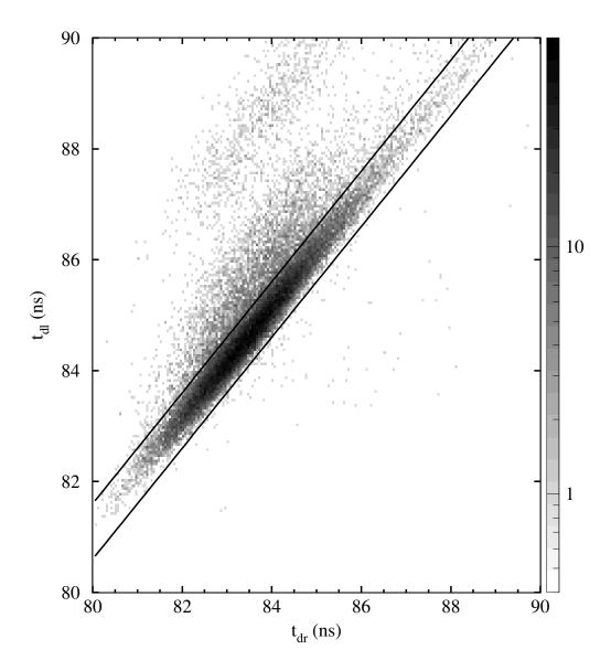
Figure 4.19: ToF of down-left PMT versus down-right PMT after travel time correction.
