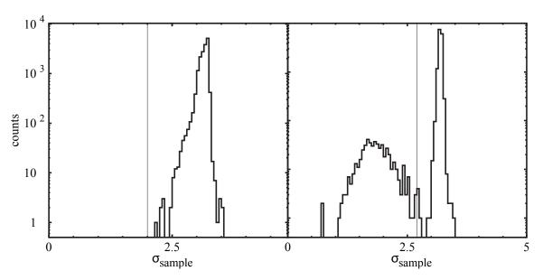
Figure 4.7: Sample width  $\sigma_{sample}$  for CRDC1 (left) and CRDC2 (right). The events to the right of the lines in each spectrum were accepted for each CRDC separately.
