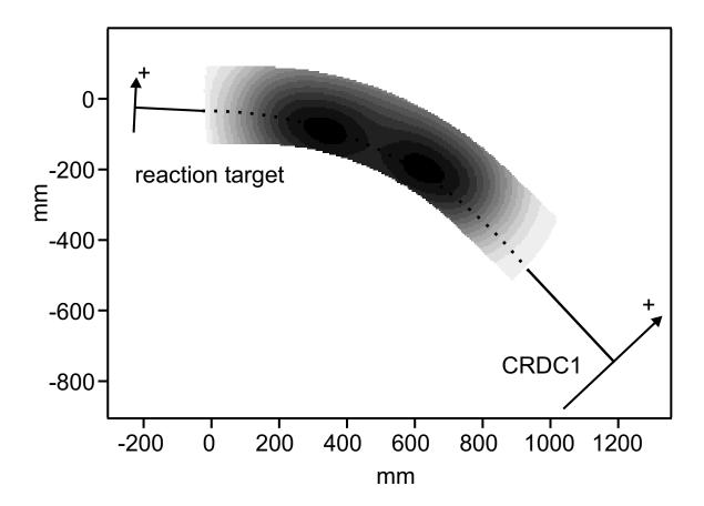
Figure 4.30: A Sweeper Magnet map with positive dispersive position marked at both the reaction target and CRDC1. The beamline and charged particle detector axis are indicated by lines perpendicular to the arrows. The dashed line represents a possible trajectory through the field. The two peaks are approximately 4 Tesla.
