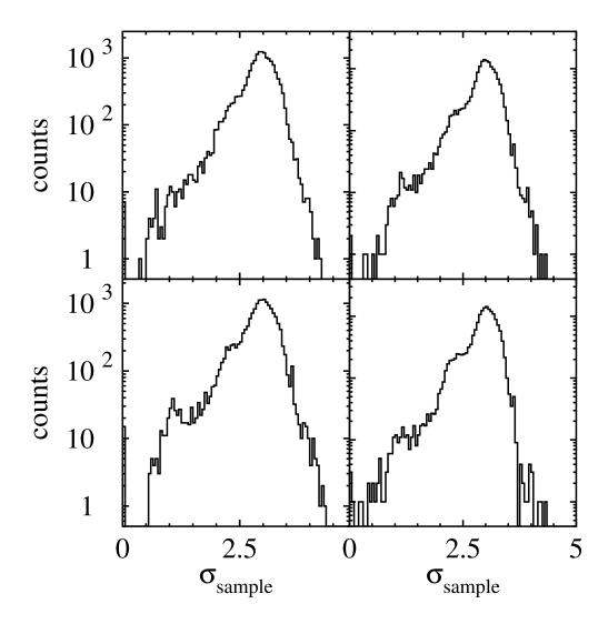
Figure 4.10: Sample width  $\sigma_{sample}$  for  $x_{PPAC1}$  (upper-left),  $y_{PPAC1}$  (upper-right),  $x_{PPAC2}$  (lower-left),  $y_{PPAC2}$  (lower-right).
