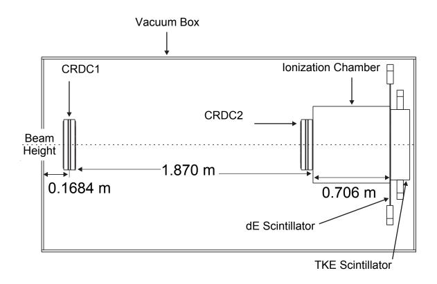
Figure 3.4: Charged particle detector layout
