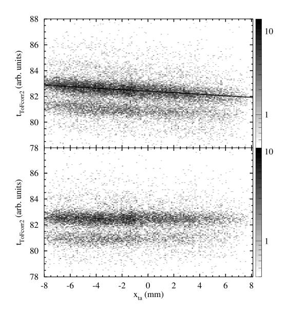
Figure 4.22: Corrected ToF  $t_{\text{ToFcorr2}}$  versus x-position at the reaction target uncorrected (top) and corrected (bottom).
