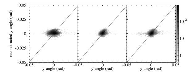
Figure 4.38: Backward reconstructed target y-angle versus measured target y-angle. Low  $B\rho$  setting (left), data-taking  $B\rho$  setting (center), and high  $B\rho$  setting (right).
