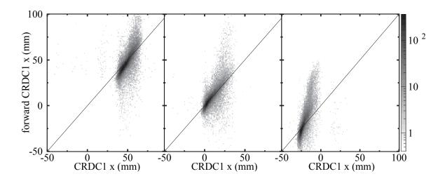
Figure 4.32: Forward-tracked CRDC1 x-position versus measured CRDC1 x-position. Low  $B\rho$  setting (left), data-taking  $B\rho$  setting (center), and high  $B\rho$  setting (right).
