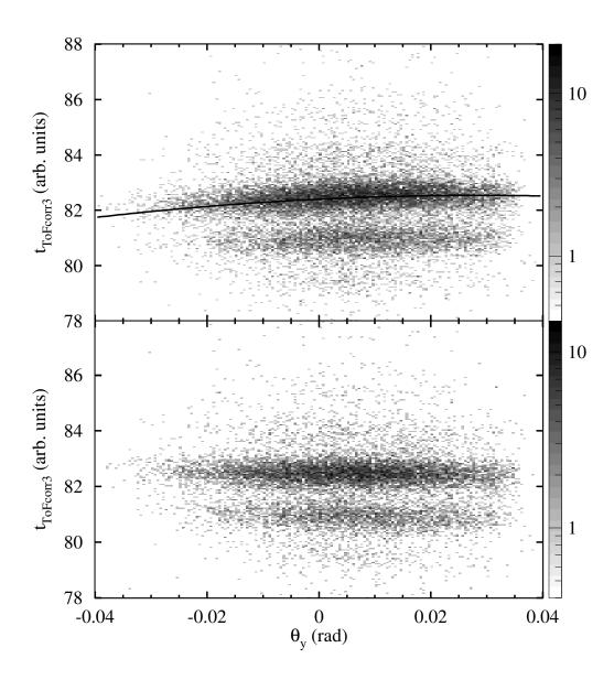
Figure 4.24: Corrected ToF  $t_{\text{ToFcorr4}}$  versus  $\theta_y$  uncorrected (top) and corrected (bottom).
