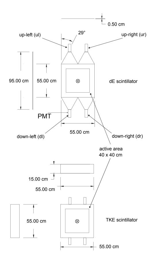
Figure 3.9: dE and TKE scintillators where the beam direction is into the page.
